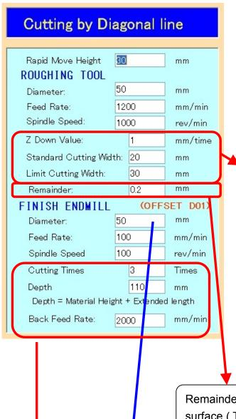
The Roughing NC data is made of the tool center.
