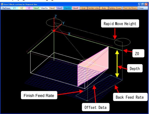
The following shows by "R CHECK" button. This figure is shown in "View2". First it goes down to the lowest Z height and returns to Z0. And it checks the movement.
